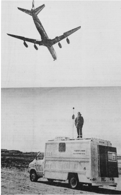
Acoustical Engineering employee measures aircraft noise on top of mobile ›Noise Measurement Vehicle‹ near Vancouver International Airport, 1973. (City of Vancouver Archives, Community Forum on Airport Development fonds, Clippings 1973–1988 folder: 578-G-7, file 5, Vancouver Sun, n.d.)
