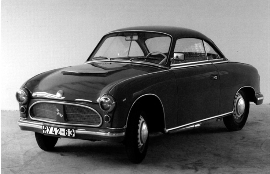
Walter Ende, P70 Coupé, Duroplast (plastic) body. Manufactured by VEB Automobilwerk AWZ, Zwickau, GDR, 1954.
